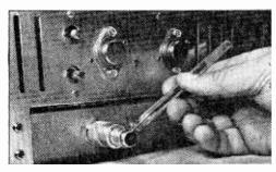
Dummy load (phantom antenna) mounts on antenna connector. It's suitable only for low-powered rigs like those for CB.
