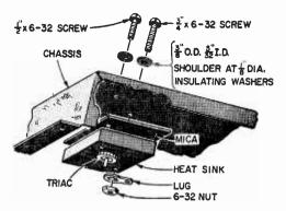
For continuous operation heat sink will be more effective on outside of chassis box—for greater heat convection the finned type of heat sink is much better.
