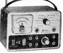
Built-in dummy load in this EICO 715 Trans/Match takes care of another test device.. Load can be switched into or out of circuit for tests.
