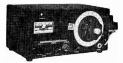
Suitable for all 2-way radio frequency checks, Lampkin Micrometer Frequency Meter has thermometer on front panel to indicate deviation of internal crystal standard. The 100,000 ohm-per-volt VOM (Lafayette Lab-Tester—below) out-performs VTVM on some ranges—without AC power.
