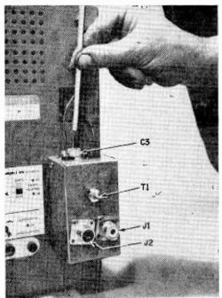
Capacitor C3 is adjusted according to the details in the text. For easier testing a dummy load (phantom antenna) can be built in—eliminating one of the coax connectors on the CB Scope Booster. Load should be shielded from transformer T1.
