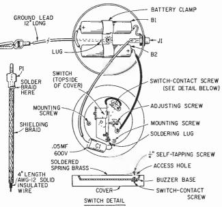
Pictorial diagram (at left) shows how parts are arranged in top and bottom sections of circular container. Batteries should be wired in series.
