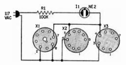
The circuit (above), is simple but you must remember it won't check all of the tubes—filaments on many 5-volt rectifier tubes are pins 2 and 8.
