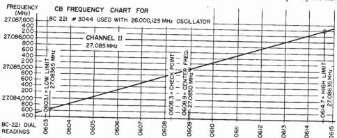
Frequency chart like that above will have to be individually made for each channel. Charts are not interchangeable with other BC-221s (or LMs) or the FO-1 oscillators.
