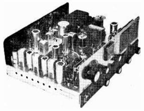
output) meter is provided along with a remote speaker jack. Though it covers 50 to 52 MHz (the popular segment of 6 meters), the dial has a special mark to indicate the American CW—only segment from 50 to 50.1 MHz.
