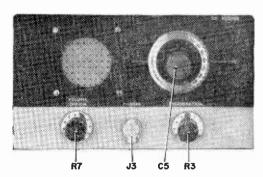
Front panel of the completed receiver is professional looking. Tuning knob for C5 can be replaced with a vernier drive for easier tuning on the communications bands.
