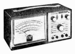
Moving on to our Dodge, which had a tendency to "konk-out" whenever the air conditioner was turned on, the EICO 888 showed that the added load of the air conditioner compressor was dropping the idle speed by 50 rpm. A quick touch-up corrected this problem, though it didn't tell us why the outfit that installed the air conditioner hadn't made this adjustment in the first place.
