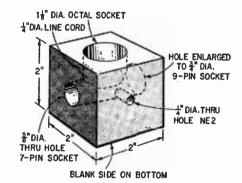
If you're not sure of your carpentry, drill the  $\frac{1}{4}$ -in. holes from each side to the center and drill the  $\frac{1}{8}$ -in. hole past center to be sure of having all other holes bore into it.
