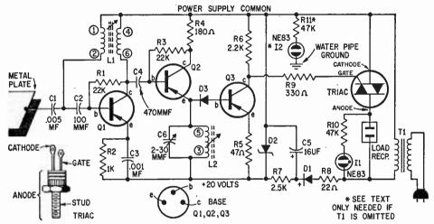
Circuit of TRIAC capacitance switch is not tricky and T1 makes it safe even though there is little chance of a dangerous shock passing through capacitor C1 to metal-plate sensor.
