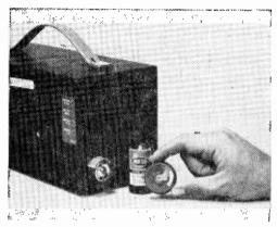
Sticker on rear of cabinet indicates the location of calibration controls on side, above battery opening—which is closed, with cap (in hand), just like a flashlight.
