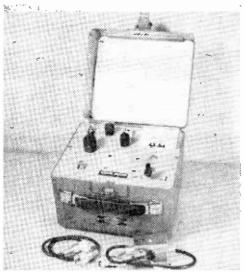
Designed for CB servicing this C12B Frequency Meter is a self-contained unit that also indicates modulation percentage and power output with built-in dummy load. Price includes 23 crystals. Unit is another made by International Crystal.
