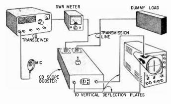
Setup for checking the CB rig's percentage of modulation requires considerable equipment—SWR meter, Dummy load (to replace antenna), and scope. Size of CB Scope Booster, as shown here, is greatly exaggerated in size. All interconnections should be made as short as possible for testing.
