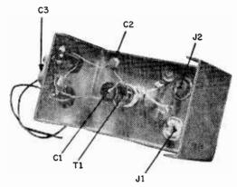
Internal view of the CB Scope Booster shows heavy-wire jumper between J1, J2 and 3-turn coil (L1) added to make T1.
