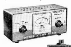
Desk-top Power and SWR meter (above) is model TM-58 from Lafayette. Inline Transicheck is made by New-Tronics. Can be easily mounted on wall, between the CB transceiver and roof-top antenna, near rig.
