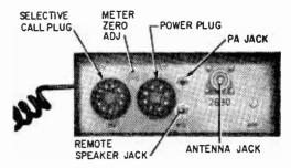
Rear apron of transceiver shows location of jacks and plugs. Internal speaker is disconnected when remote jack is used.
