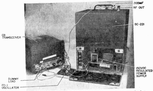
Rear view of setup for frequency check of CB transceiver shows power supply that replaces battery pack of original frequency meter design and also powers FO-1 chassis.
