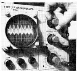
This high-quality scope is too expensive for anyone but the professional. Added feature of Textronix scope are plug-in subassemblies that multiply usefulness.
