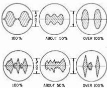
Scope patterns show the modulation tests made with tone (top and below) and voice. Voice patterns keep jumping around on the screen and percentage of modulation can only be estimated. Accurate measurements can be made when using tone modulation.
