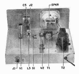
spaced as shown. The plug-in connector for the coil (J2) is mounted on an aluminum bracket approximately 1 in. high by 3/4 in. wide. Use a single hole mounting type jack with ceramic insulation.
