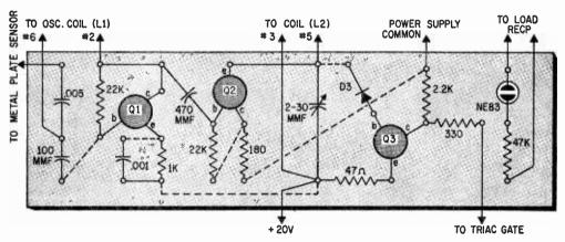
Component-board layout shows position of small components. Use spaghetti (plastic tubing) on the base lead of Q1 and Q3 to prevent short circuits. Dotted lines are wire connections on under surface of the perforated phenolic board used as chassis.
