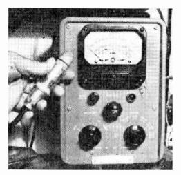
For extremely accurate AC (audio and RF) measurements are made with this Hewlett-Packard VTVM. Price puts it outside the budget of the individual. It's popular in research and development work though.
