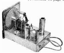
Companion to transceiver is this Knight-Kit V-107 VFO (variable frequency oscillator).
