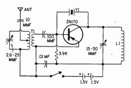
put circuit (L1) is a BCB loop antenna or loopstick. The crystal (Y1) can be a 25.96 MHz (mc) rock. By tuning the transistor receiver and leaving the converter alone, you can cover from 26.51 to 27.56 MHz—all 23 CB channels. Quality of performance depends on how close L is to the loopstick inside the transistor radio. Strong broadcast stations will still be heard on the pocket BCB radio.
